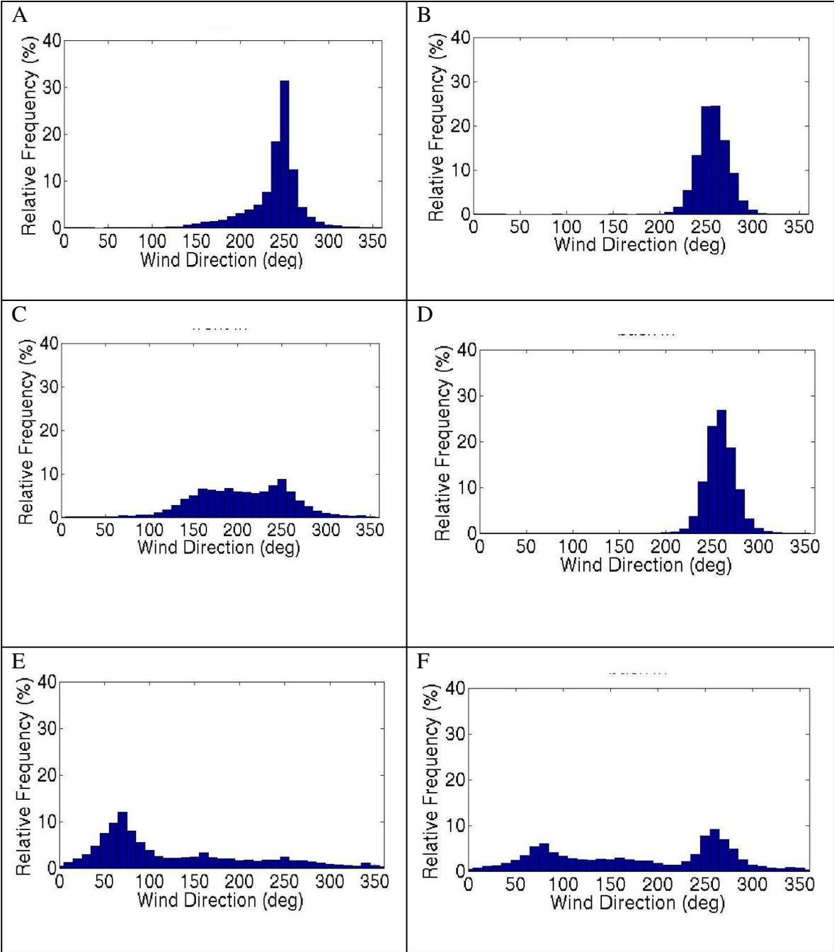
Figure 4. Statistical distributions of the instantaneous wind directions measured inside the cubes at the west-ward (a, c, e) and east-ward (b, d, f) openings (positions in-1 and in-2 respectively, notation of the sonic is the same as in Figure 2a) for flow perpendicular (a,b) diagonal (c,d) and parallel (e,f) to the openings.
