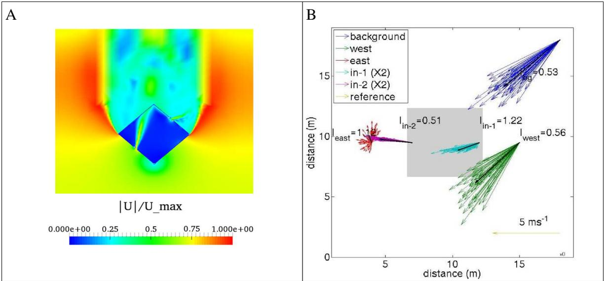
Figure 2. Normalised instantaneous velocity magnitude ( $|u|/u_{ref}$ ) on a horizontal plane at window height 3.5m for wind directions  $45^\circ$  (King et al., 2017- a). Flow conditions under background flow at wind directions  $45^\circ$  at 1-6-2015, 23:00-24:00 UTC. Sonic anemometer data are shown as 1-minute mean wind vectors. Turbulence intensities are also shown for every anemometer (b).
