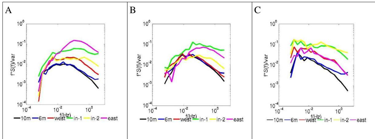
Figure 5. Frequency spectra of the wind speed under perpendicular (a) diagonal (b) and parallel (c) flow measured on 2-6-2015, 09:00-10:00 UTC, 1/6/2015 23:00 – 24:00 UTC and 4-6-2015, 11:00-12:00 UTC respectively.
