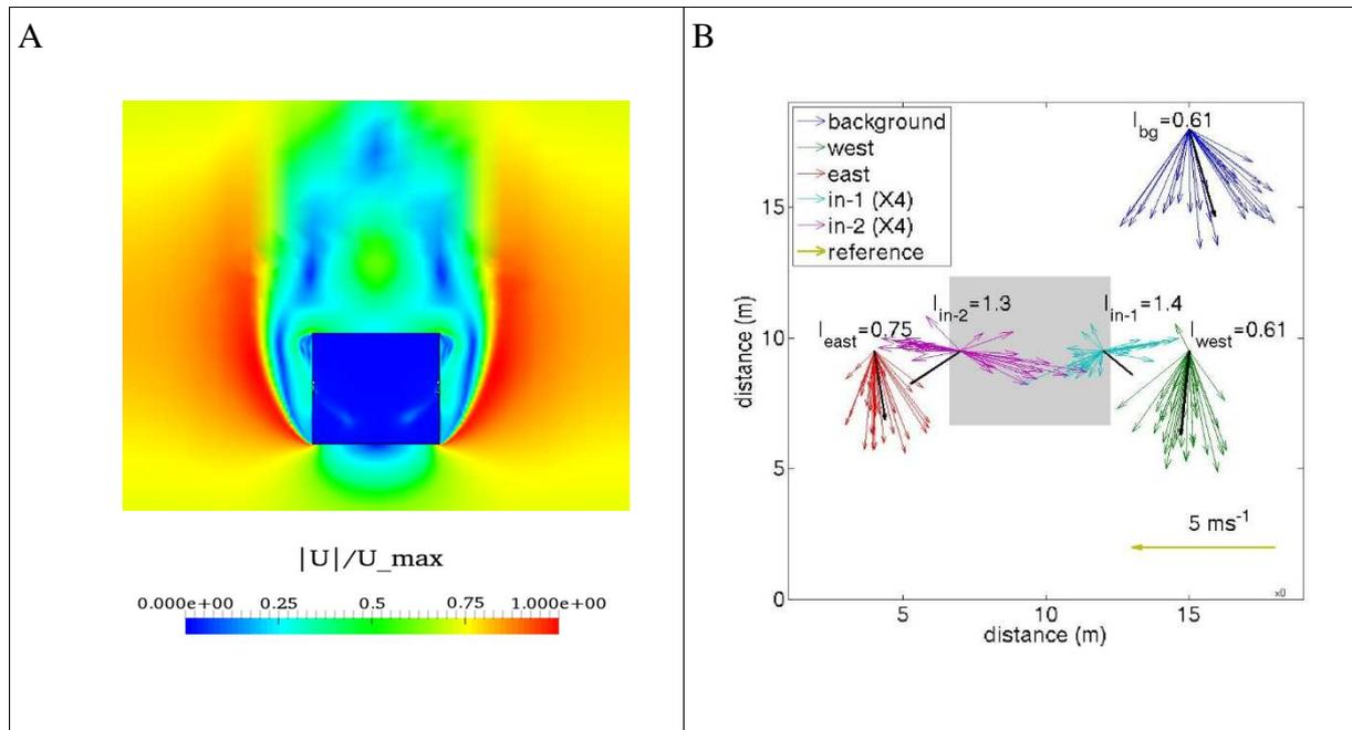
Figure 3. Normalised instantaneous velocity magnitude ( $|u|/u_{ref}$ ) on a horizontal plane at window height 3.5m for parallel flow (wind directions  $0^\circ$  King et al., 2017 - a). Flow conditions under parallel background flow at 4-6-2015, 11:00-11:30 UTC. Sonic anemometer data are shown as 1-minute mean wind vectors. Turbulence intensities are also shown for every anemometer (b).
